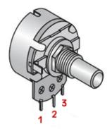
Volume Pot - Note the numbers 1, 2, 3 on the layout. Be sure to connect the right pins on the pot to the right pads on the board. +9v Ŷ Out O ο 0 Output 📂 0 1 2 3 VOLUME 494 Å •C2 • Ognd OIn Input 📂 Ō В ●C1 ● Ground
