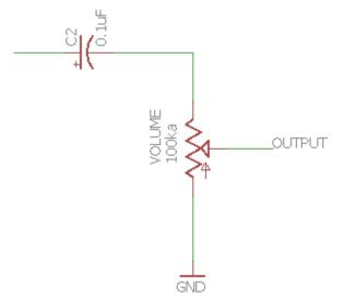
The 100nF C2 output capacitor blocks DC and provides simple high pass filtering. C2 and Volume Pot create a high pass filter.
