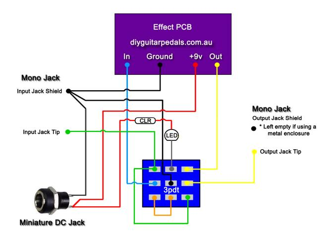
"CLR" = Current Limit Resistor. This resistor (included with your LED and bezel controls the brightness of the led and stops the LED from blowing. Also note the flat side of the LED, examine your LED closely you will note it physically has a flat side. This is the negative side of the led as pictured above
