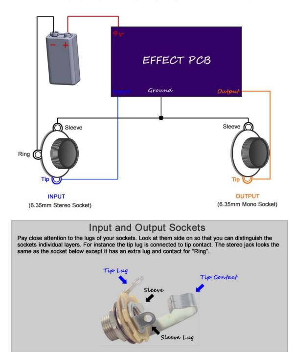
**Note,** you can still test your effect with 2 mono jacks, just combine the negative of the battery with the ground input sleeve connection. A DC Jack will also work for a power source, replace the battery above with a dc jack.
