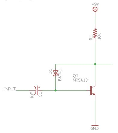
The Q1 transistor just needs to be high-gain (h<sub>FE</sub> of 5,000 minimum per the MPSA13 datasheet). The lower the h<sub>FE</sub> value on the selected Q1 transistor, the less saturation and fuzz will occur and the higher the h<sub>FE</sub> value, more saturation and fuzz.
