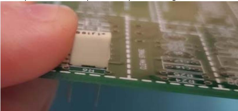
Orientation of “which way is up” doesn’t matter, so you can install them either way. After installation and soldering, do not forget to clip the remaining legs from the PCB.
