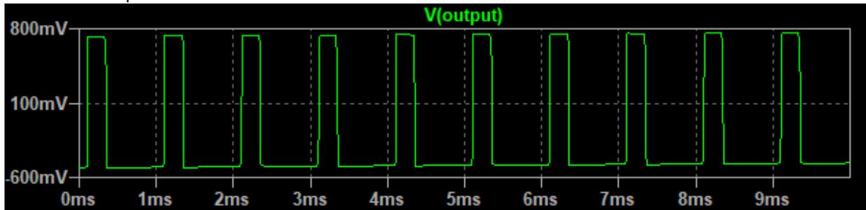
As the R4 resistor is lowered to 22K, the waveform starts to change as seen with the positive 800mV side.
