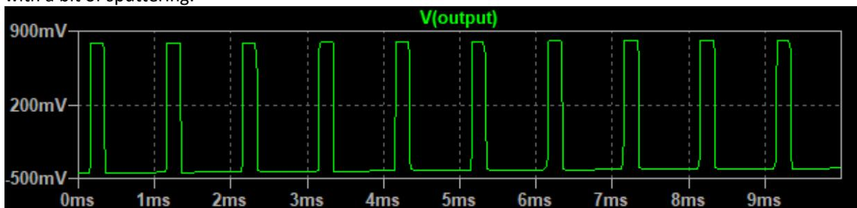
As the resistor reaches towards 1M, the sputtering becomes more apparent, which typically isn't desirable.
