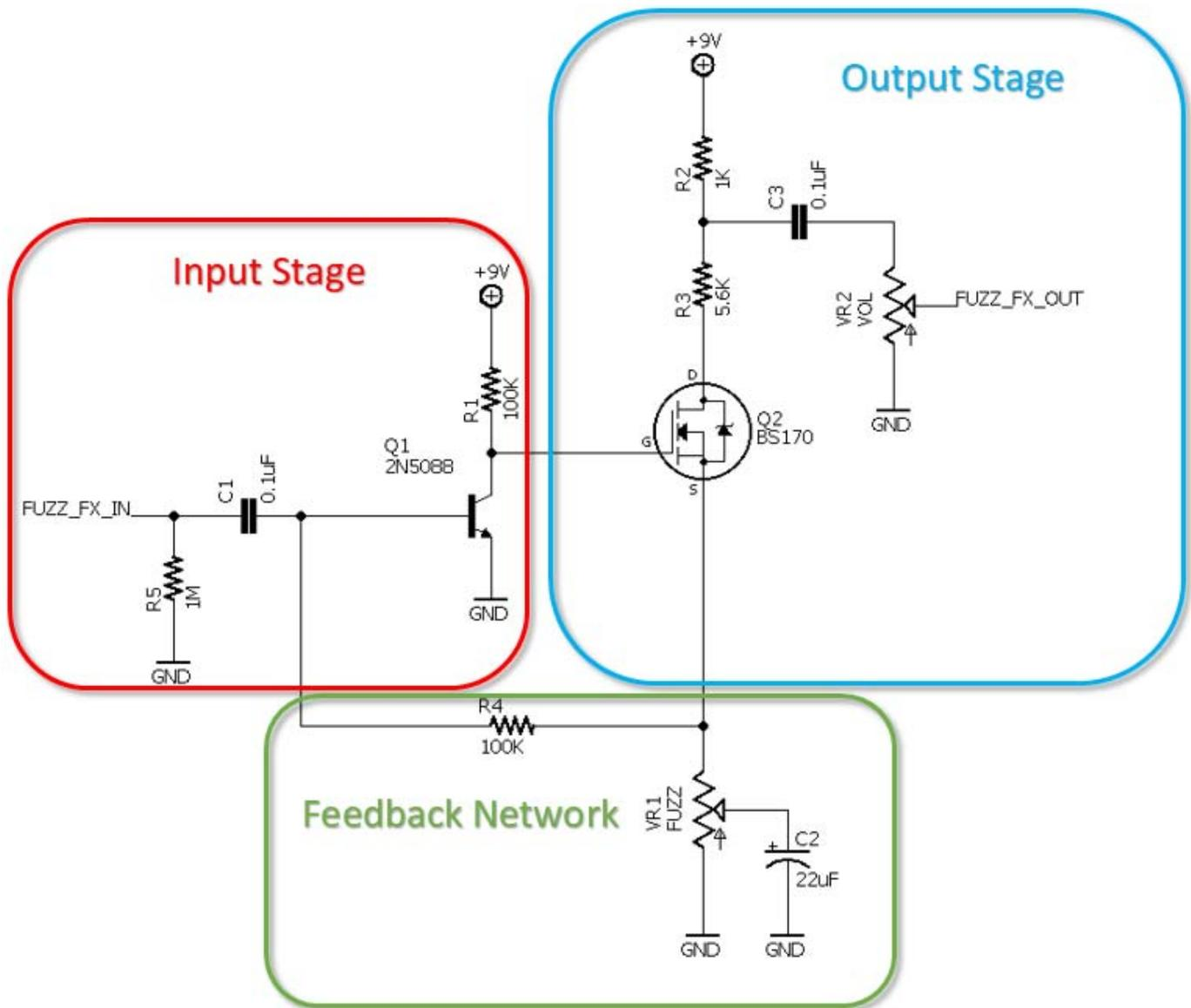
The circuit is designed around a BJT-MOSFET pair for gain.
