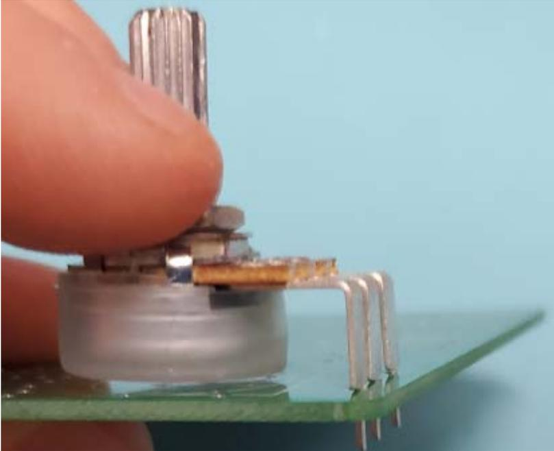
This pedal can utilize 16mm pots. These are typically installed on the backside of the PCB and uses the included washer and jam-nut to mechanically secure the PCB to the enclosure via a strategically drilled hole on the enclosure. Orientation of potentiometer is preferred to line up the knob on the silk screen with the knob of the potentiometer.
