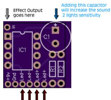
There are 2 outputs, Led+ and Led- is one output. Each output can take a minium of 2 Led's. Experiment with more Led's. Maximum will vary depending on your Led's forward voltage.
