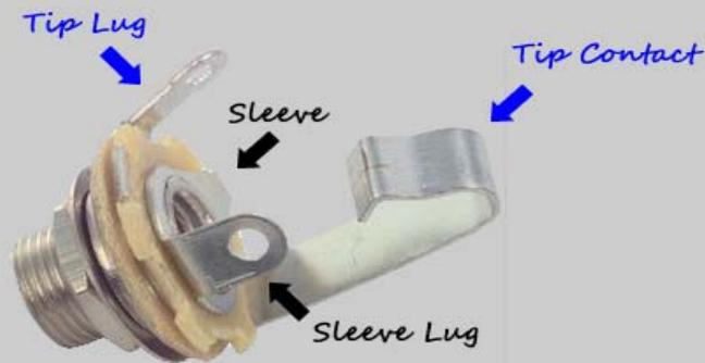
**Note**, you can still test your effect with 2 mono jacks, just combine the negative of the battery with the ground input sleeve connection.
