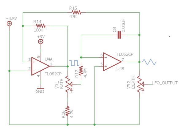
The first operational amplifier in the chain generates the square wave, while the second operational amplifier generates the triangle signal.
