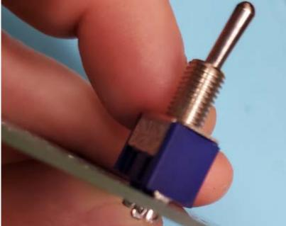
These are typically installed on the backside of the PCB and uses jam-nuts to set the "height" of the actuator and to mechanically secure the PCB to the enclosure via a strategically drilled hole on the enclosure. Orientation should not matter with most switches.
