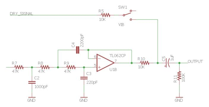
The R5 resistor is used to sum in the dry signal with the wet signal coming out of the op amp. By breaking this connection via SW1, only the wet vibrato signal makes it out, changing the pedal from a chorus (wet and dry signal combined) to a vibrato pedal (only the wet signal).
