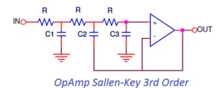
A common configuration for BBD based designs is to use a 3rd order Sallen-Key, implemented using a passive 1st order RC filter + a 2nd order standard Sallen-Key.
