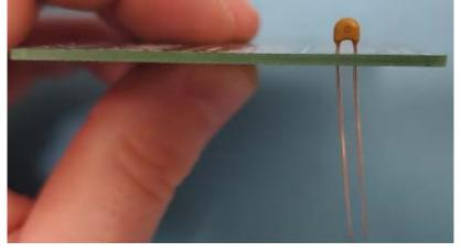
Orientation of "which way is up" doesn't matter, so you can install them either way. After installation and soldering, do not forget to clip the remaining legs from the PCB.
