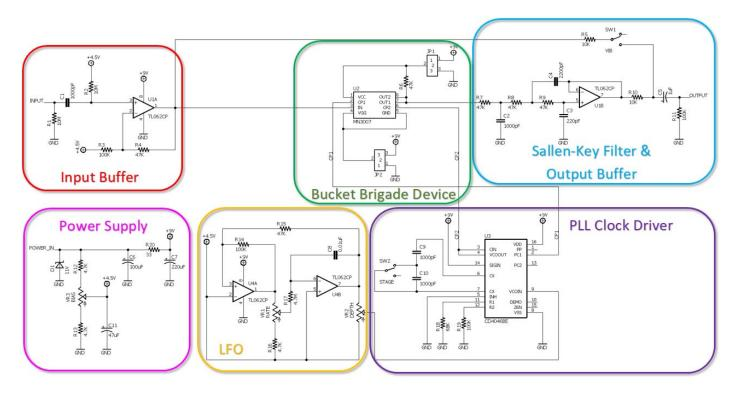
The circuit is designed around the MN3007 or MN3207 1024 stage BBD (U2) and the CD4046 PLL clock driver (U3). The input and output circuits use the dual op-amp TL062 IC, while the LFO is implemented with the help of an additional TL062LP op-amp.
