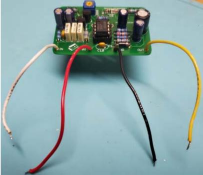
These can be installed at the very end, but in some situations, installing them before potentiometers are soldered in place can be advantageous. Colored wire doesn't change the properties, but using color codes for hot and ground wires, like red being hot, and black being ground, are common place. Typically, stranded hook-up wire, AWG 24 or 22 is used for this task. Using wire strippers, strip away about 1/8" (3mm) of the wire from either end and then using a soldering
