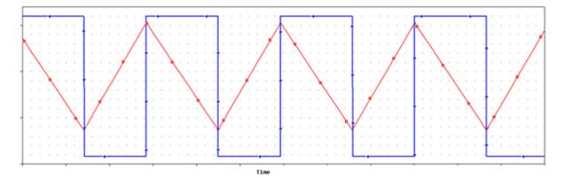
The first op-amp is in a threshold detector in positive feedback Trigger-Schmitt configuration. The oscillation frequency can be calculated following the formula of the Triangle Oscillator by Ron Mancini:
