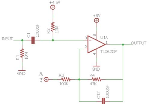
The TL062 op amp is a low power op amp that generates little electrical noise making it suitable for audio applications.
