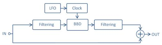
Before and after the BBD delay action, there are some stages needed to avoid signal degradation: Pre/De-Emphasis and Anti-Aliasing/Reconstruction filters.
