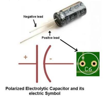
After installation and soldering, do not forget to clip the remaining legs from the PCB.
