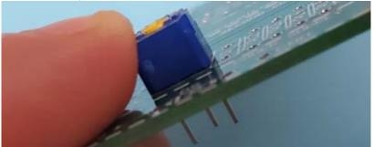
These devices have holes on the PCB that will allow them to only be soldered in one way.
