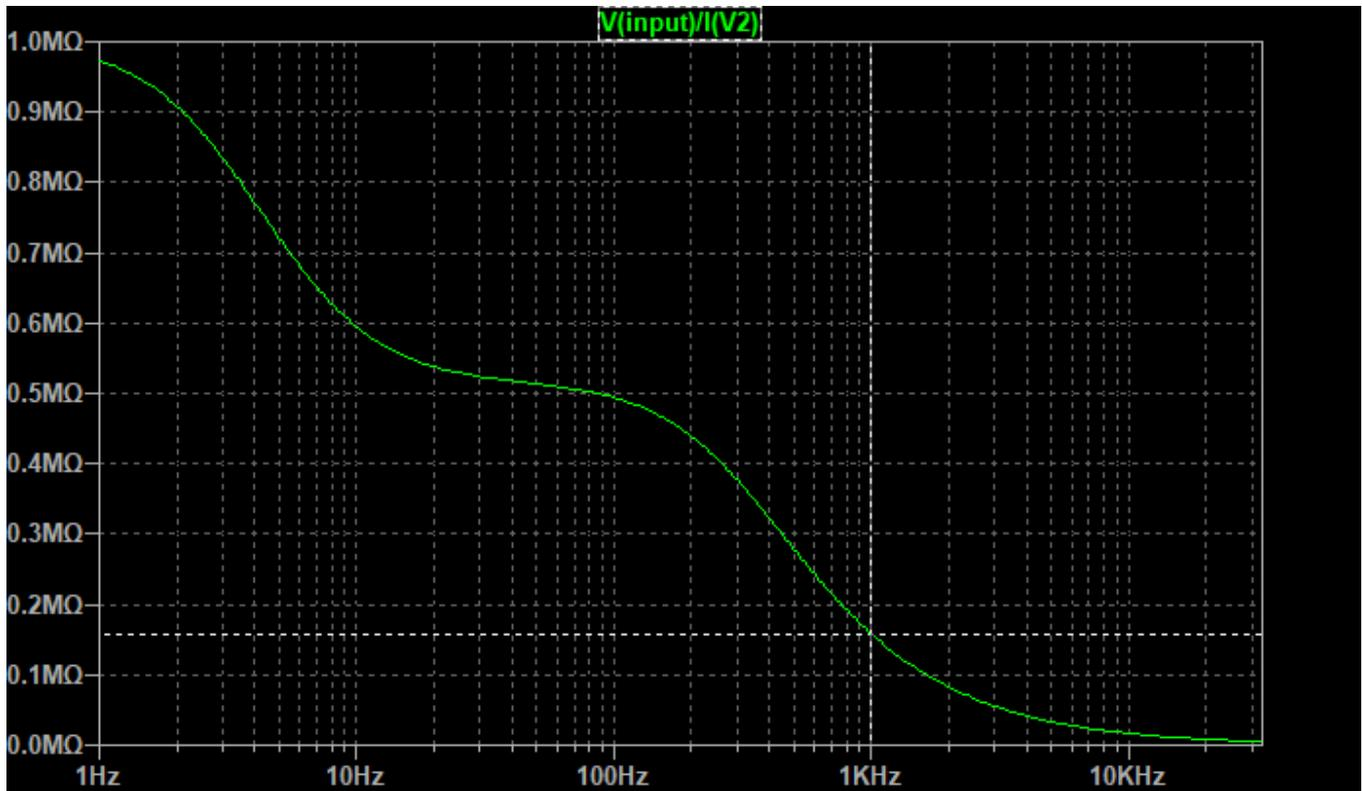
Lowering the capacitance of C2 improves the input impedance as the 1KHz mark. For example, if C2 drops to 470pF, at 1KHz, the input impedance raises to 284KΩ
