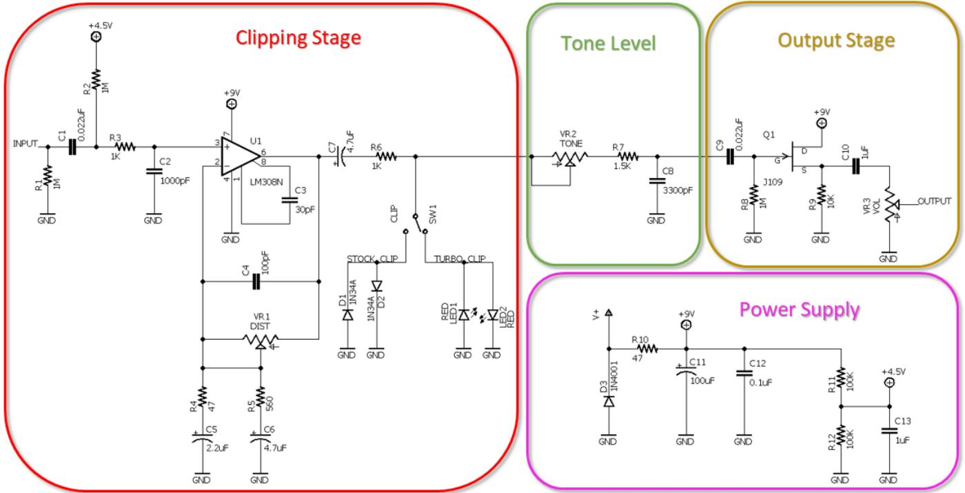
The design is based on the LM308 single op-amp. The distortion is produced using a variable gain circuit with diodes clipping the waveform. The distortion stage is followed by a tone filter and an output buffer stage that ends up with a tone control.
