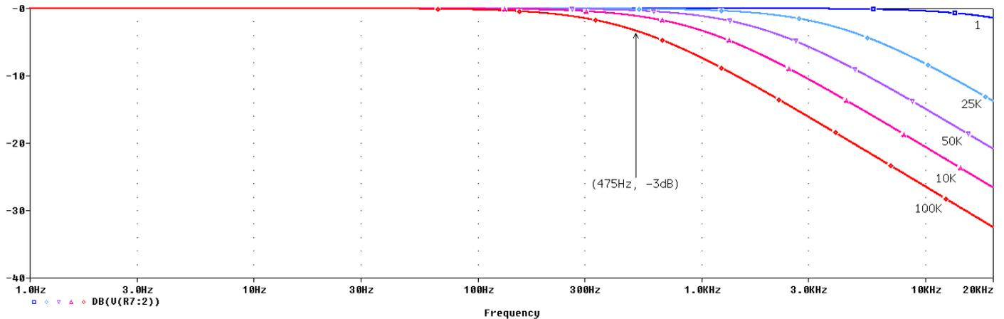
The range of the filter is pretty wide, being able to sweep almost all the audio spectrum from 475 Hz to 32 kHz. The Tone Control combined with all the other filters placed in the pedal will create a mid-hump, to be analyzed in the Frequency Response Section.
