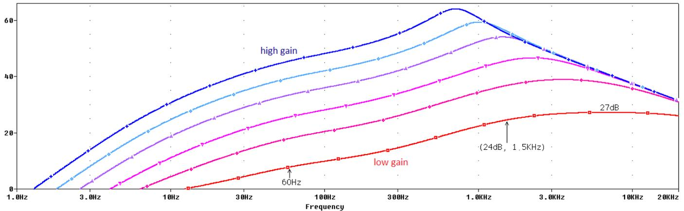
In the image above, the response of the Clipping Stage is shown. The signal is band limited in high and low frequencies. This mid hump around 1 kHz helps to keep the guitar sound from getting lost in the overall mix of the band.
