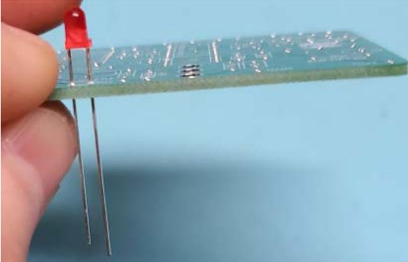
These devices will have a silk screen notch to indicate an orientation. Make sure the flat side on the PCB matches the LED's flat cathode when placing on the PCB.
