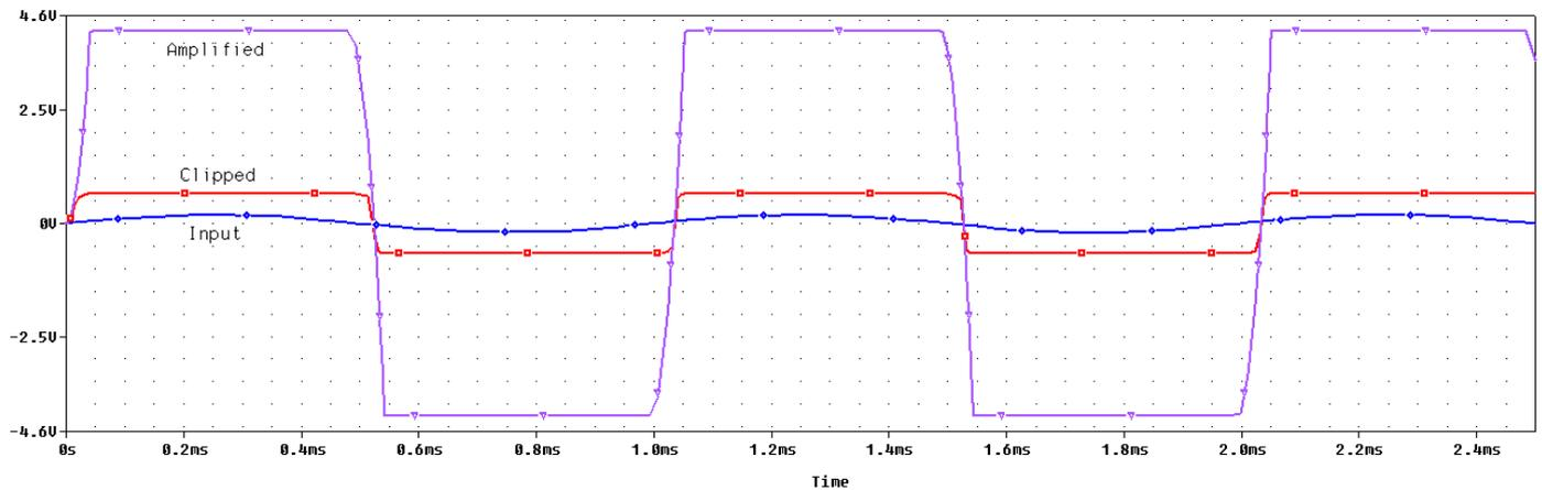
In the above graph, the input signal is represented in blue color. This original signal will be amplified by the op-amp until the power supply limits (line represented in purple). After the voltage gain, the diodes will clip the signal to  $\pm V_F$ .
