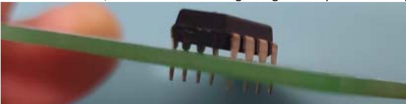
Orientation of “which way is up” will be indicated by a notch on the silkscreen on the PCB and a dot or bar on the actual IC itself. Do make sure they match.
