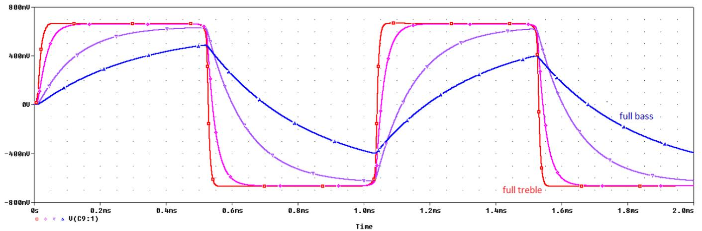
The clipped waveform will be affected by the low pass filter, as shown above, creating a shark fin shape as the tone control is dimed.
