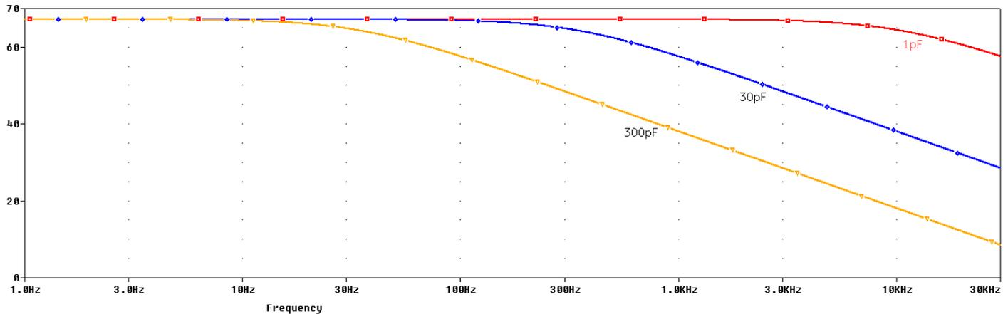
The above image shows again how the high frequencies are attenuated, using a 30pF cap for C3. Using bigger/smaller caps the Bandwidth and Slew Rate will be reduced/improved.
