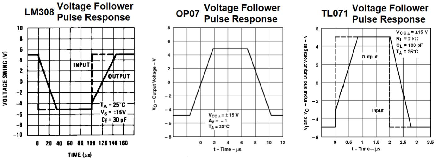
In the image above, the slew rate of the LM308 and OP07 is shown together with the TL071 (standard op-amp used in stomp boxes) for comparison purposes. The TL071 slew rate is 13V/μs while the LM308 and OP07 are 0.3V/μs. This means the LM308 and OP07 are 40 times slower, which in turn indicates how slow is the op-amp inside this pedal will be.
