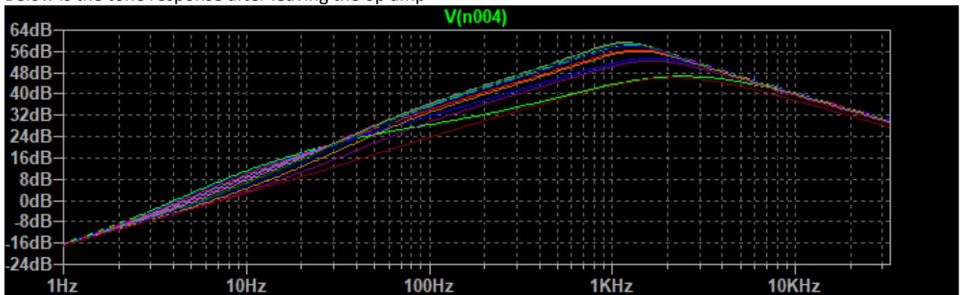
Combined with the RC filters going into the op amp, ones in the negative feedback loop the overall tone response seems focused at around a 1.17 KHz hump across the full sweep of the distortion knob.
